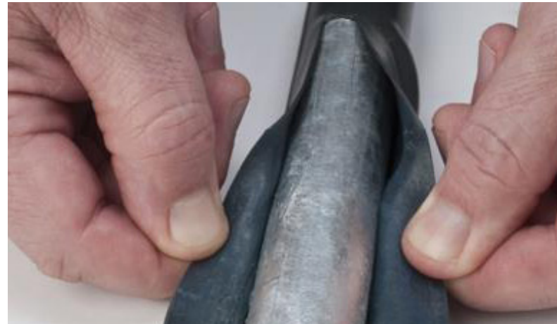
PVC coated conduit specimen where the coating adhesion has failed. This conduit sample was exposed for approximately two days in the Hot Water Immersion Test. Once the cuts are made, the PVC coating is easily removed by pulling the coating by hand and exposing the galvanized steel conduit.
