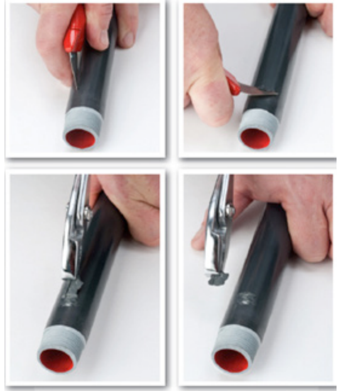
Physical testing shown above confirms successful adhesion of the PVC coating to the substrate.
