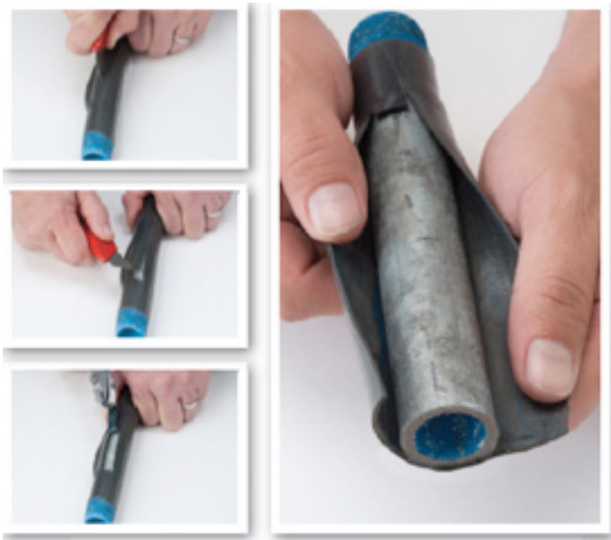
Physical testing confirms major adhesion failure of external PVC coating.
