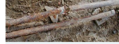
Rigid metal conduit placed underground at a renovation of a convenience store with fueling islands, it was revealed that the conventional conduit that runs to the pumps had suffered greatly from corrosion. To learn more about corrosion and how to eliminate the cost associated with replacement of product due to failure – attend Corrosion College.
