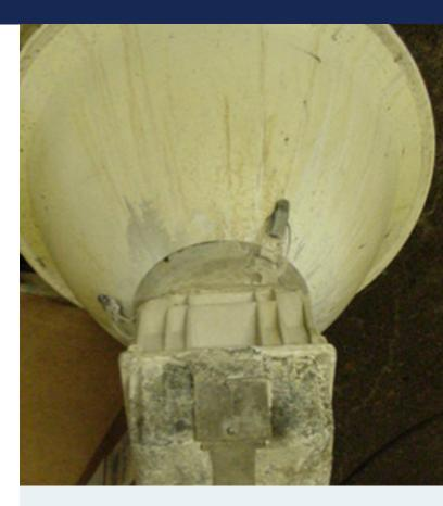
Corrosion discovered on lighting fixture by an electrical engineer in a food manufacturing plant shortly after graduation from Corrosion College. Immediate replacement of the fixture eliminated any potential danger of corrosion flakes falling into the food being processed directly below.
